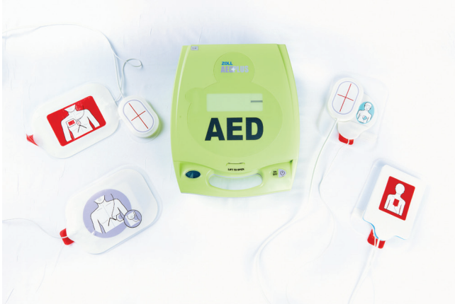
Figure 4-9 | While AEDs work the same regardless of the patient's age, the pads or setting used for children and infants differ.
