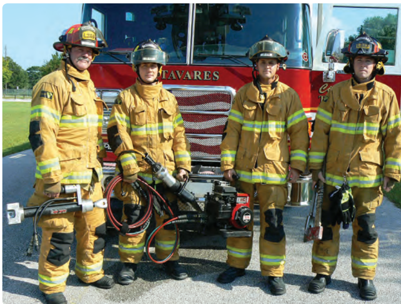
Fig. 28-7: Extrication tools used to access patients include hand tools, pneumatic tools, hydraulic tools, cutters and rams. Photo: courtesy of Ted Crites.
