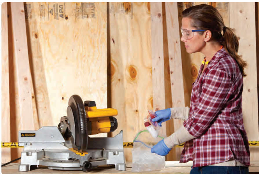
Fig. 20-12: Wrap a severed body part in sterile gauze, seal it in a plastic bag and put the bag in an ice and water slurry.
