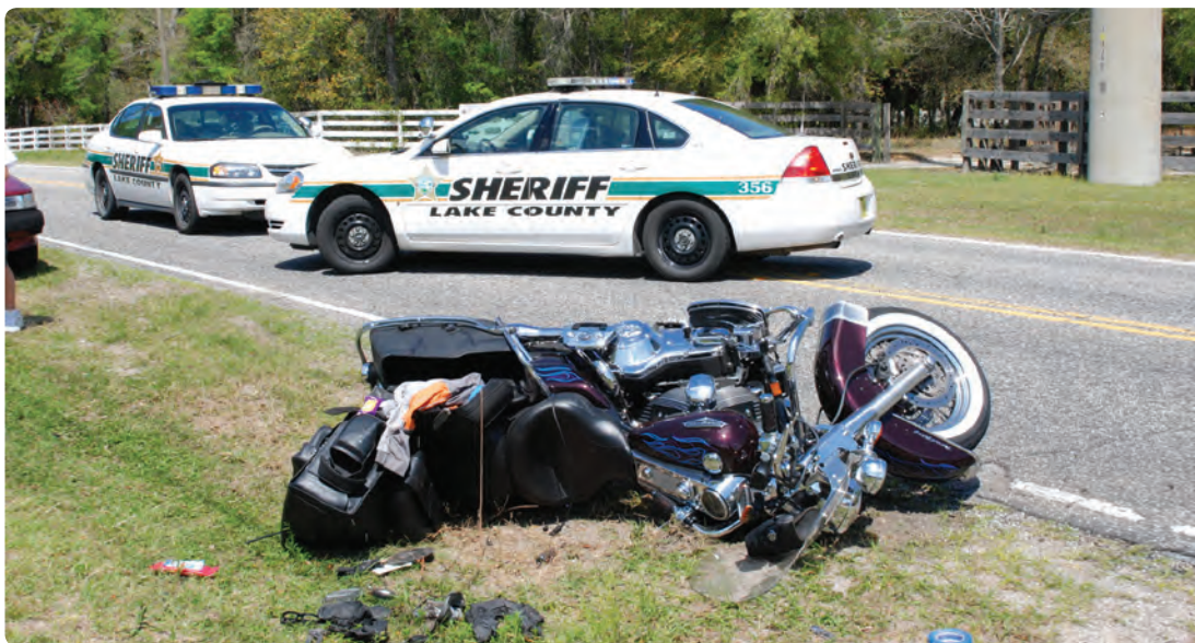
Fig. 28-2: Blocking is a method of controlling traffic in which emergency vehicles are positioned to create a physical barrier between the emergency scene and the flow of traffic. Photo: courtesy of Captain Phil Kleinberg, EMT-P.
